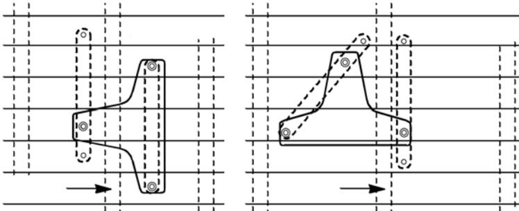
Access is normally achieved by removing a section of floorboard adjacent to the fixing area large enough to allow the insertion and positioning of the bars. All floorboards taking any part of the load should be securely fastened down to the joists with 4" (100mm) countersunk wood screws. The final installation should be tested according to the manufacturers recommendations.
